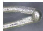
[그림 1] Present industrial temperature sensor manufacturing method and example of element deterioration (Sentech E & G Co., Ltd.)
