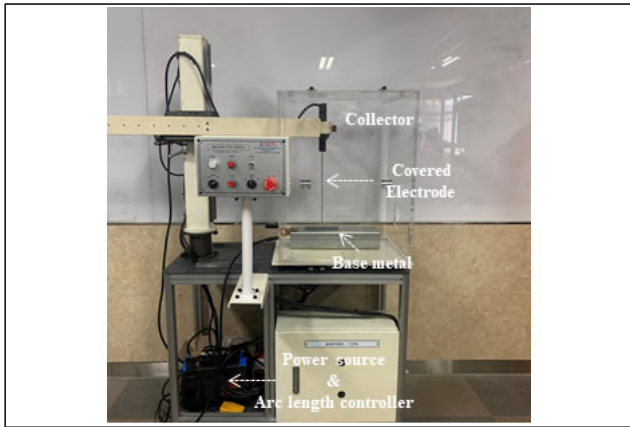
[그림 2] The Schematic Diagram of welding equipment setup showing the SMAW electrode and Base Metal
