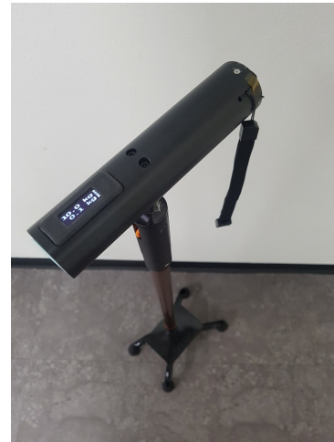
[Fig. 1] A weight-support feedback cane (WSFC). WSFC can be used in a mono cane and in a quadripod cane by switching the cane's legs.
