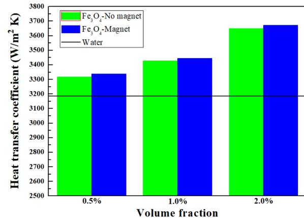
[Fig. 4] Heat transfer coefficient for water and  $\text{Fe}_3\text{O}_4$  nanofluid with various volume fractions considering without and with magnetic effect
