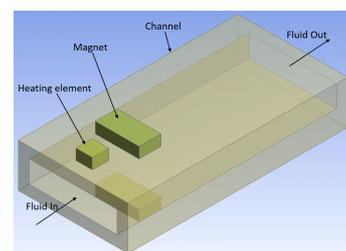
[Fig. 1] Three-dimensional geometry of minichannel with water and nanofluid flow
