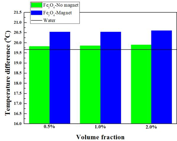
[Fig. 3] Temperature difference for water and  $\text{Fe}_3\text{O}_4$  nanofluid with various volume fractions considering without and with magnetic effect
