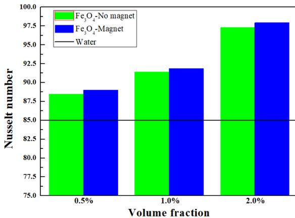
[Fig. 5] Nusselt number comparison for water and  $\text{Fe}_3\text{O}_4$  nanofluid with various volume fractions considering without and with magnetic effect
