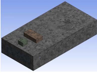
[Fig. 2] Meshing configuration for considered computational domain
