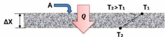
[그림 677] Heat conduction through a section of asphalt pavement
