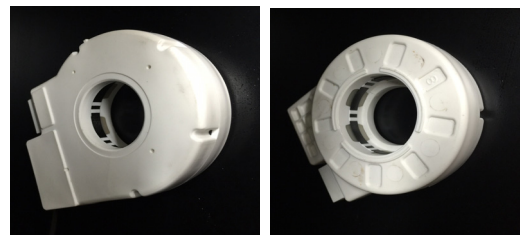
Fig. 16. Experimental results of insert injection molding using the inserted part with holes.
