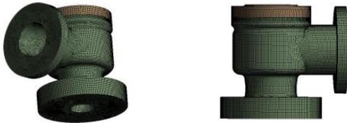
Fig. 5. Computational Mesh of Structural Analysis
