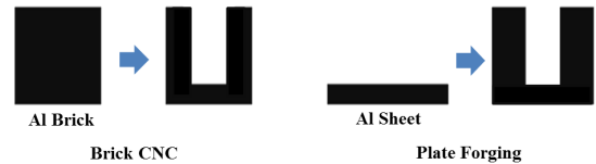
Fig. 2. Comparison between Brick CNC and plate forging
