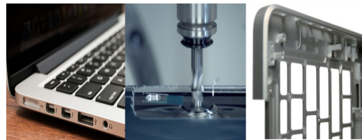
Fig. 1. Brick method of Apple's Macbook Pro (CNC machining and laser finishing)
