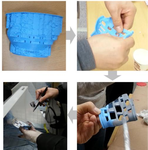
Fig. 7. Post-processing performed on the 3D printing
