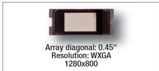
Fig. 3. Applied DMD(DPL4500) in This Paper (Texas Instruments)
