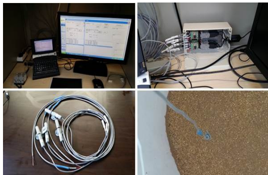
Fig. 2. Temperature/humidity sensor and data server
