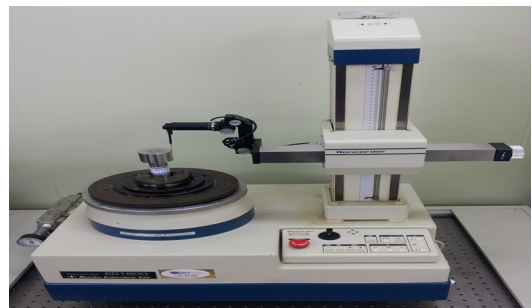
[Fig. 8] Circularity testing machine(EC1800)
