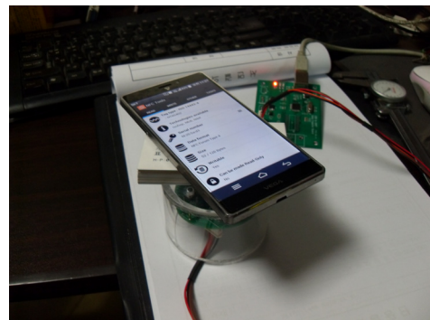
[Fig. 12] Sensing Distance & Sensing Rate Measurement
