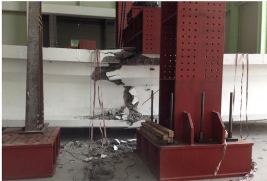
[Fig. 13] Test specimen failure
