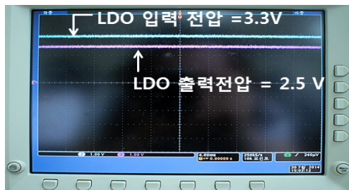
[Fig. 13] Measured results of the LDO output.
