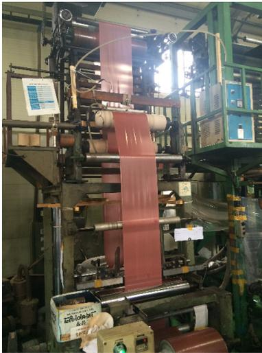
Fig. 4. Manufactured film through the blow process.
