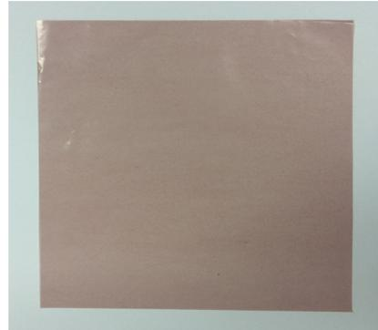
Fig. 5. Manufactured film through the Blow process.
