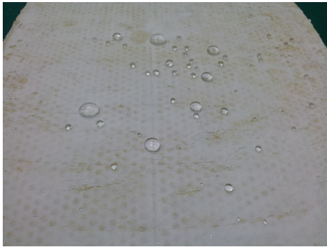
Fig. 8. Hydrophobic characteristic on glass wool
