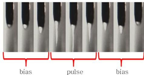
Fig. 4. Cone-jet mode of EHD pump system
