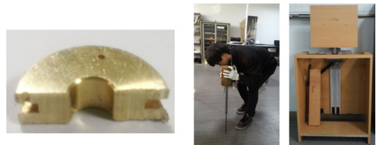
Fig. 18. Pipe type orifice piston and experiment
