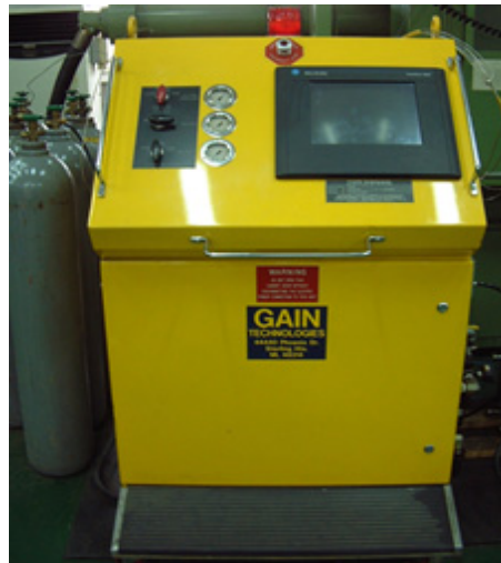
Fig. 5. GAS Injection of Unit
