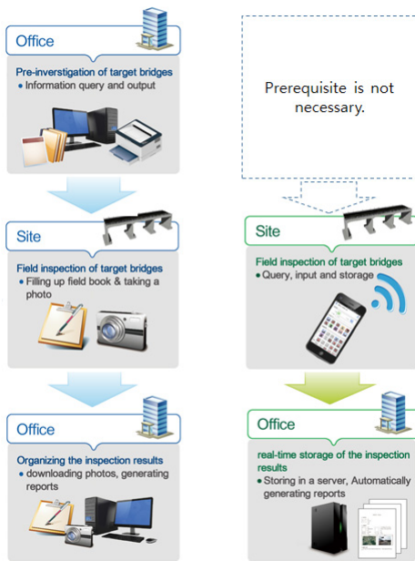
Fig. 1. Comparison of existing method and proposed method in bridge inspection
