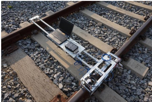
Fig. 6. Rail surface roughness measurement with automatic running platform
