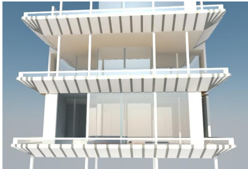
(b) Isometric view of inclined balcony system
