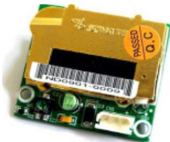
Fig. 5. CO<sub>2</sub> sensor in TREMS
