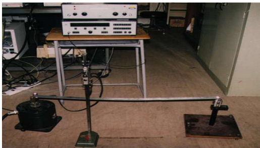
Fig. 6. Experimental setup for modal tests.
