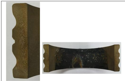
[Fig. 23] Metal flow of completed part after a hot ring rolling and heat treatment
