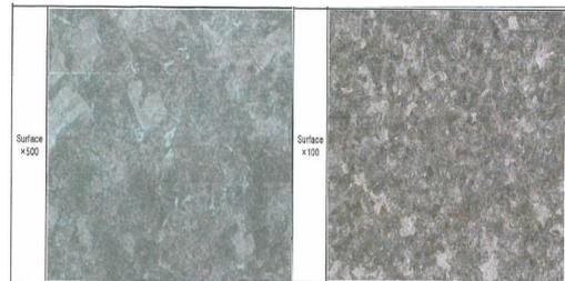
[Fig. 25] Micorstructure after heat treatment (Q/T)
