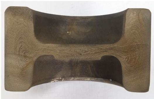
[Fig. 22] Metal flow for a blank in finishing process
