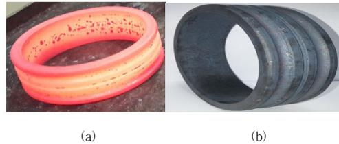
[Fig. 20] Finished test samples (a) after hot ring rolling (b) in cold state
