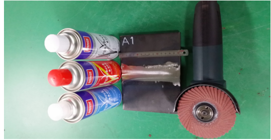
[Fig. 8] Penetration weld inspection testing equipment
