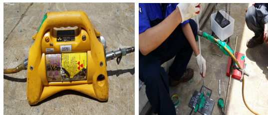
[Fig. 9] Photo of the shooting scene and radiographic inspection test equipment
