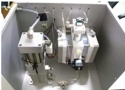
[Fig. 8] Developed PSPI D&P system apparatus unit
