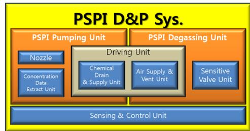
[Fig. 2] Structure of PSPI D&P system
