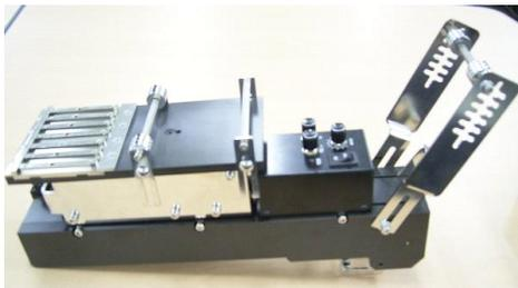
[Fig. 1] Stick Feeder used by a Vibration
