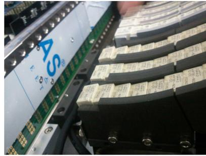
[Fig. 2] Relay are not horizontally stand
