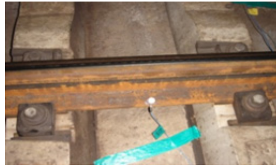
Fig. 5. Vibration measurement of track components
