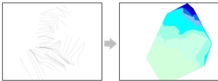
③ Calculating Inundation Area and Depth by the Difference Topography DEM in Flood Level DEM
