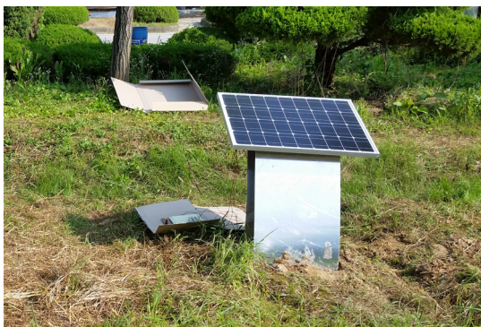
Fig. 1. Heat storage experiment equipment of solar cell module
