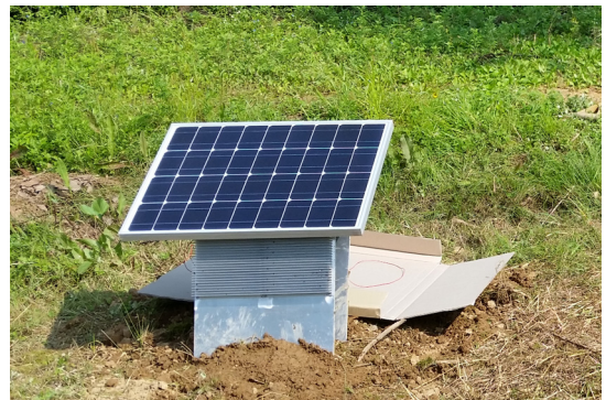
Fig. 2. Experimental equipment to air radiation and geothermal conduction of solar cell module.
