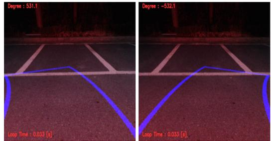
Fig. 22. Parking guideline according to handle steering angle
