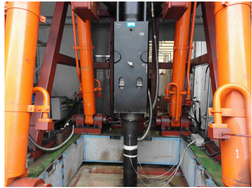
Fig. 8. Picture of hydraulic breaker test in KIMM
