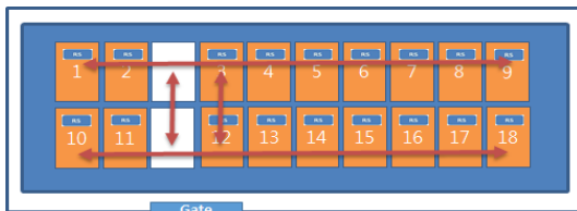
Fig. 8. Vertical Circulation System
