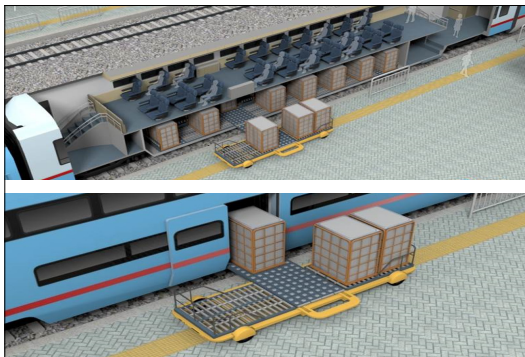
Fig. 1. Concept of Passenger-Baggage Hybrid Train
