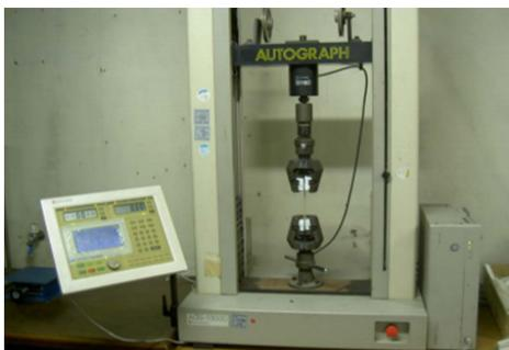
Fig. 2. UTM for Tensile Strength
