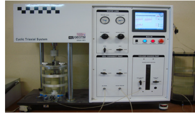
Fig. 3. Consolidation undrained triaxial compression experiment
