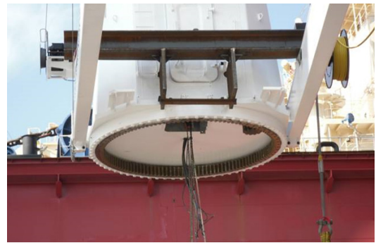
Fig. 2. Temporary fixing jig
