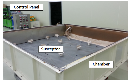
Fig. 9 Equipment set-up of performance test for susceptor.
