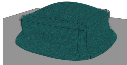
Fig. 11. Deformed shape at the moment of maximum load (@0.01sec)
