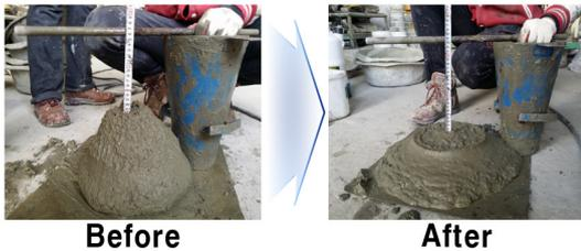
Fig. 3. Improving material property using form concrete
