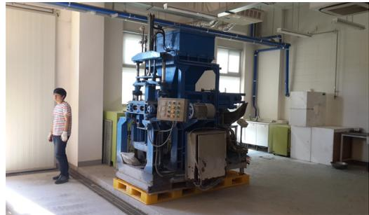
Fig. 1. Concrete block making equipment
