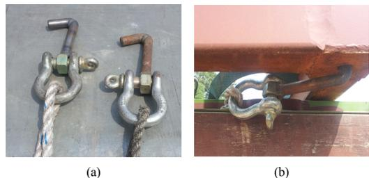
Fig. 1. Fixing equipment of existing for transporting the unit module
