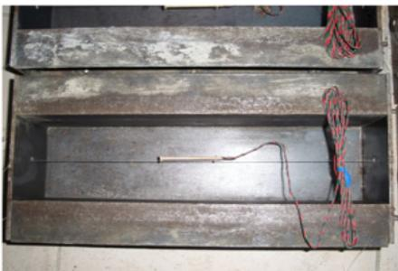
Fig. 4. Shrinkage length change tester for concrete
