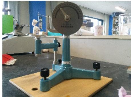
Fig. 2. Surface tension measuring device for liquid
