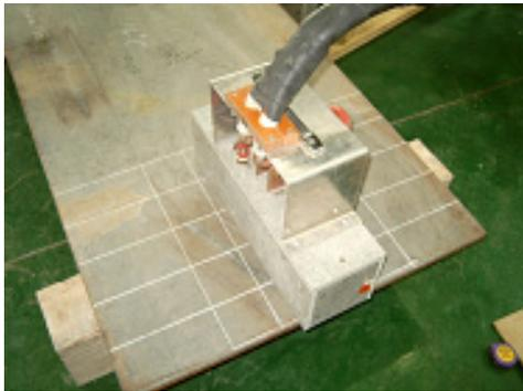
Fig. 11. Arrangement of induction heating machine for experiment
