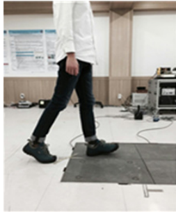
Fig. 4. Ground reaction force measurement
