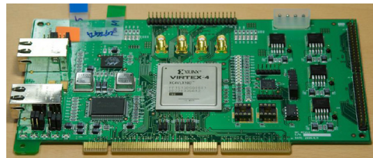
Fig. 4. Photograph of the FPGA prototype board
