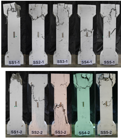
Fig. 7. Failure patterns of square columns
