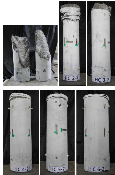
Fig. 10. Failure patterns of circular columns
