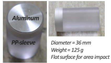
Fig. 6. Projectile for impact test
