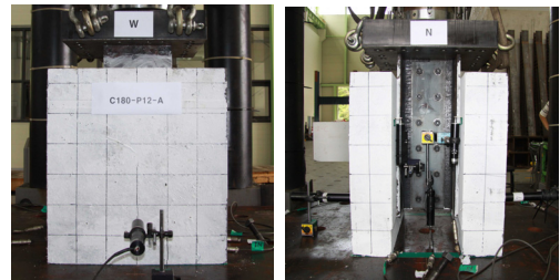
Fig. 5. Views of push-out test
